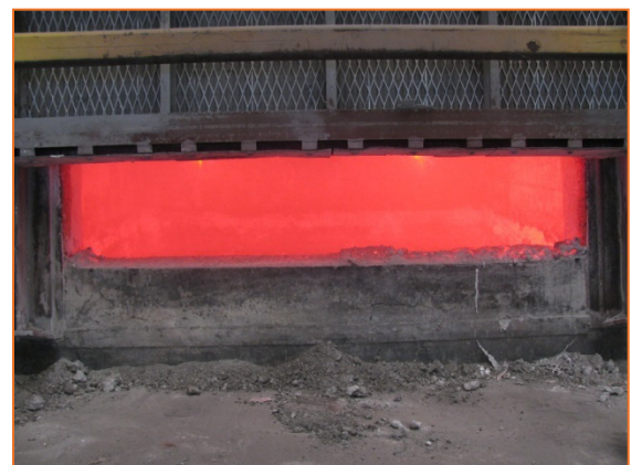
ARMORMAX® 70 AC sill after 10 months service
